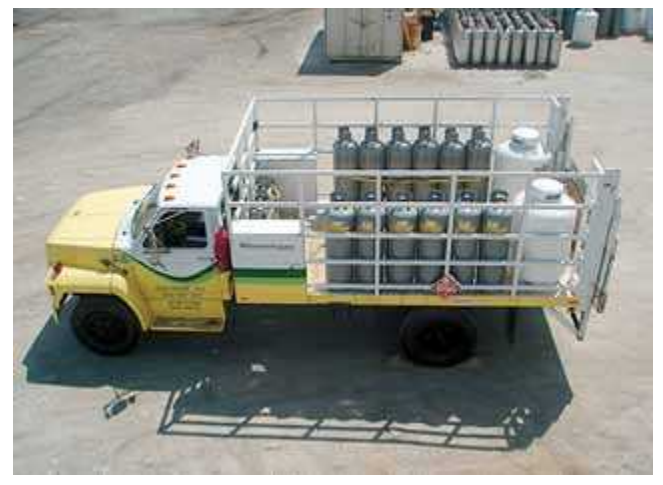
Cylinders in an open portable container cargo vehicle (delivery truck). (Courtesy of Eastern Propane Corp.)
