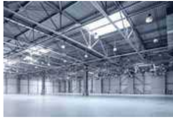
(b) Type II construction
