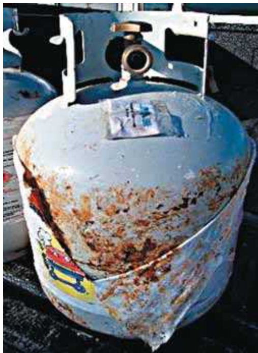
Cylinder showing corrosion under a sleeve (sleeve removed). (Courtesy of Richard Fredenburg, North Carolina Department of Agriculture and Consumer Services)
