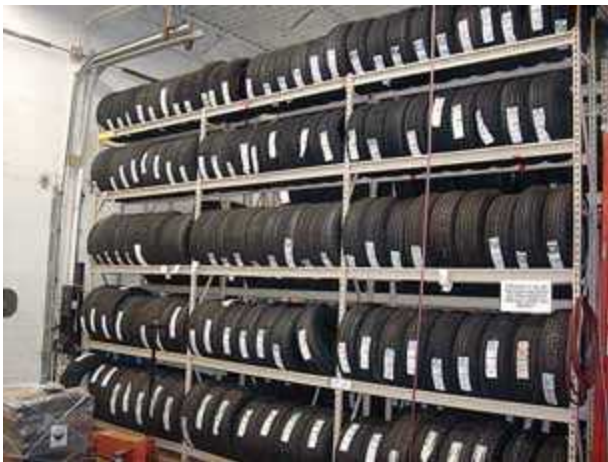
On-tread tire storage on racks.
