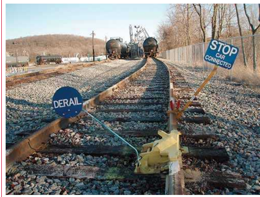
"Stop" and "Derail" signs on a track. (Courtesy of Eastern Propane Corp.)
