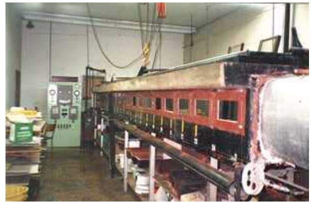
ASTM E84 tunnel test apparatus. (Photo courtesy of Herbert Blenstein)
