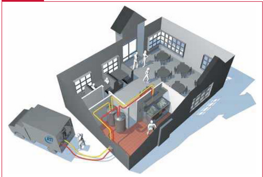
Example of a combined cooking oil storage system that handles fresh and used cooking oil. (Courtesy of Restaurant Technologies, Inc.)
