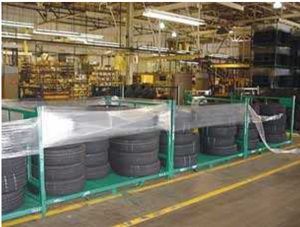
On-Side Tire Storage on Portable Racks. (Courtesy of Ford Motor Company)
