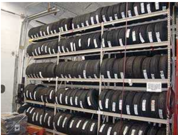
On-Tread Tire Storage on Racks.
